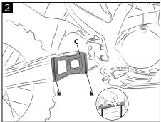
Place the support (C) and close the zip ties (E) identifying the anchor points.
