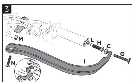
**Fix the bar (I) to the handlebar using the expander (H), the insert (L), the spacer (C) and the screw (G) as shown in the figure. Fix the bar to the bracket using the bushing (M) and the screw (N).**
