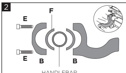
**Mount the bracket (B) on the handlebar using screws (E) and use the spacers (F).**
