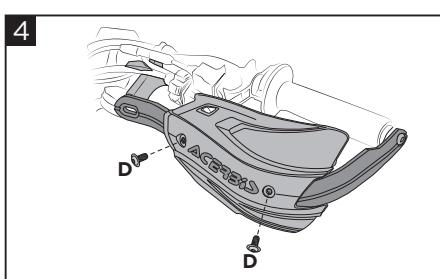
**Assemble the cover to the bar using the screws (D).**
