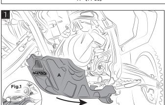
With force, push the skid plate (A) back towards the rear as indicated with the arrow. Make sure that the hook on the back of the skid plate is securely placed up and over the rear frame support
