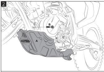
Secure the Skidplate (A) to the frame by tightening the bolts (B) on both sides.
