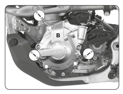
Remove 3 OEM ignition cover bolts exactly as indicated in the image above. Attach the X-Power ignition cover with the remaining 3 (C) bushings and the 3 stock ignition cover bolts and tighten to the OEM torque settings in the owners manual.
